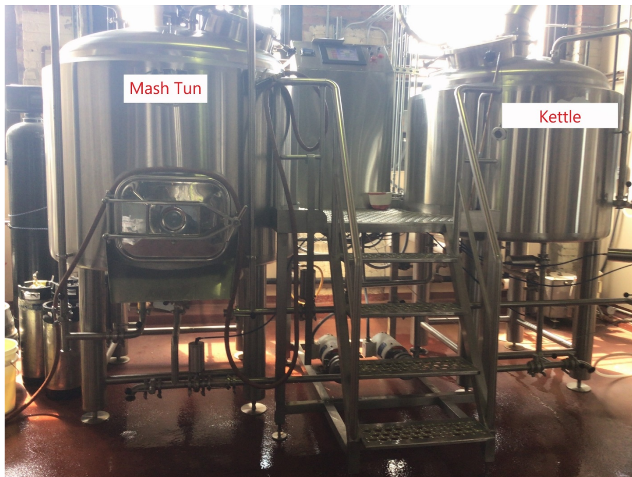
Figure 2 Mash tun and kettle at Lo-Rez Brewing
